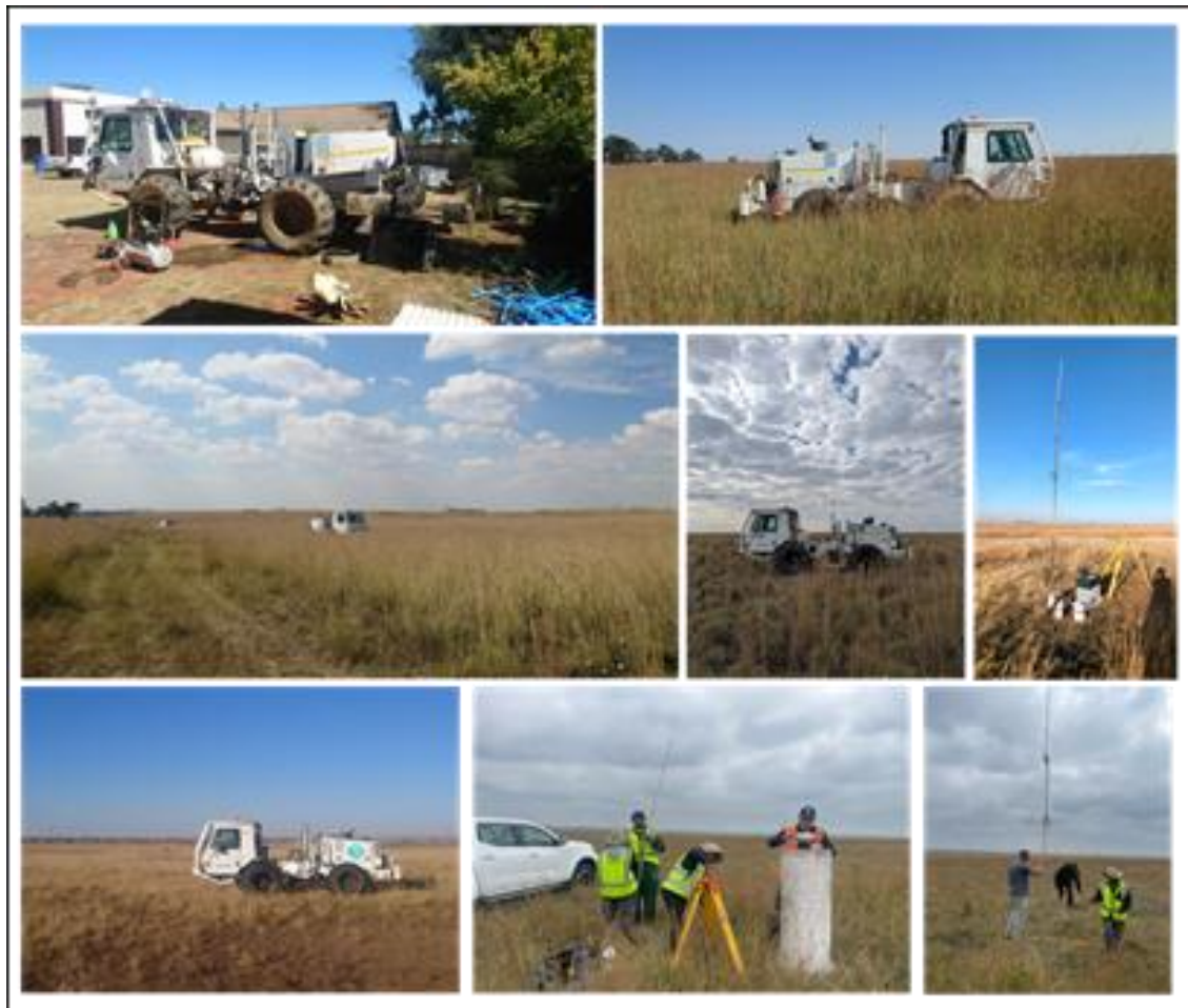
Figure 1-5 Images of 12-ton source truck (minivibrator) provided by EIMS (2023).
