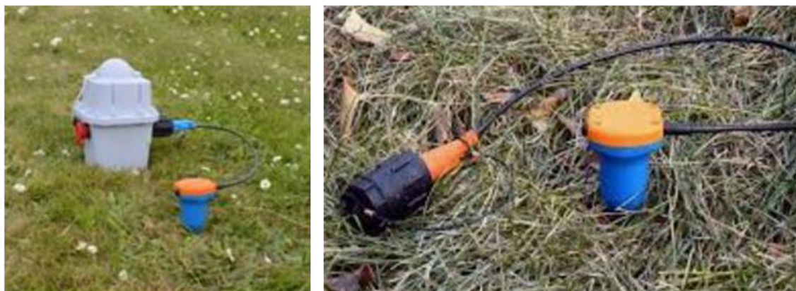
Figure 1-6 Geophone unit to be utilised for seismic acquisition provided by EIMS (2023)
